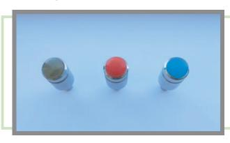
Supply of standard piston/stamp with the diameter of 10mm, 20mm and 30mm. Additionally, different piston/stamp will be especially made for different temperature ranges depending on the model of
